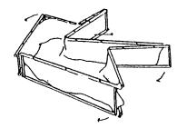
Place collection pool on a hard and level surface. A tarp may be used over rough ground to protect the pool liner.
