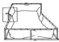
Extend each side of pool until hinge locks. Secure non-hinged side of pool with one locking pin. (Standard Collection Pool only).
