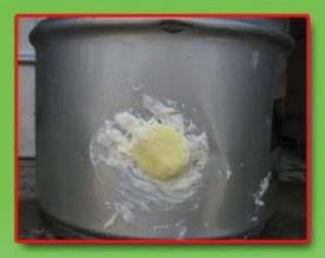
Part #SPG GOLF BALL PLUG is an inch and a half round, polyurethane impregnated, water activated foam plug used to temporarily stop the flow from a leak in anything from a pipe to a tanker, to a railcar-even a boat! It is initially pliable to insert into a void and quickly expands and hardens to fill the void-it can even be applied below the water line.
